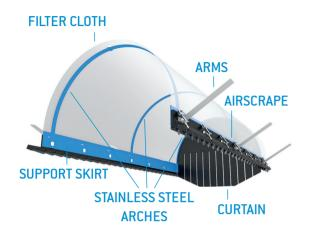
Installed above the conveyor belt, the filtering cloth retains dust particles created by conveyed material, while remaining permeable to circulating air. The filter cloth is specifically designed to retain dust particles and is durable, maintenance-, contact- and energy-free. It is easy to install and can be manufactured to any size.
